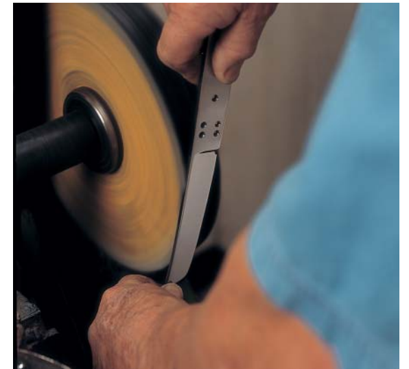
McNabb’s class focuses on the stock-removal process of knife-making, in which a blade is cut and shaped from a flat of steel. The process involves cutting out the shape of the blade with a band saw, shaping it with belt grinders (above) and then polishing it.
