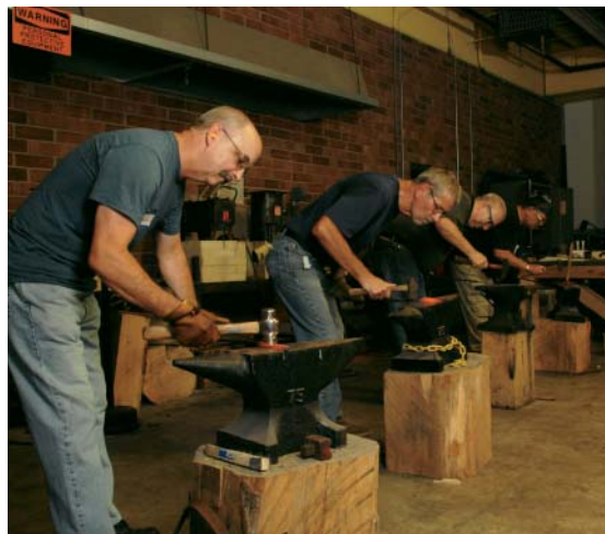
Montgomery Community College in Troy offers beginners a chance to learn to make knives themselves. Batson's class (right and opposite page) teaches students how to properly heat and hammer-forg a blade from a simple carbon steel rod.
