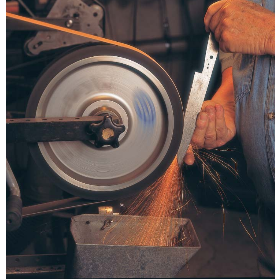
McNabb’s class focuses on the stock-removal process of knife-making, in which a blade is cut and shaped from a flat of steel. The process involves cutting out the shape of the blade with a band saw, shaping it with belt grinders (above) and then polishing it.
