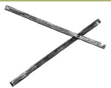
Figure SK3. Setting tool
