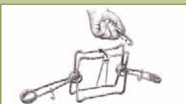
Figure BV5b. Using safety gripper
