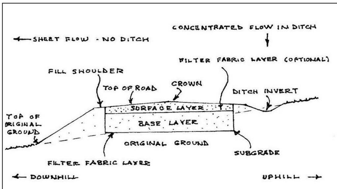
Figure 2 – Typical Road Cross-Section – Canaan, NH Highway Department
