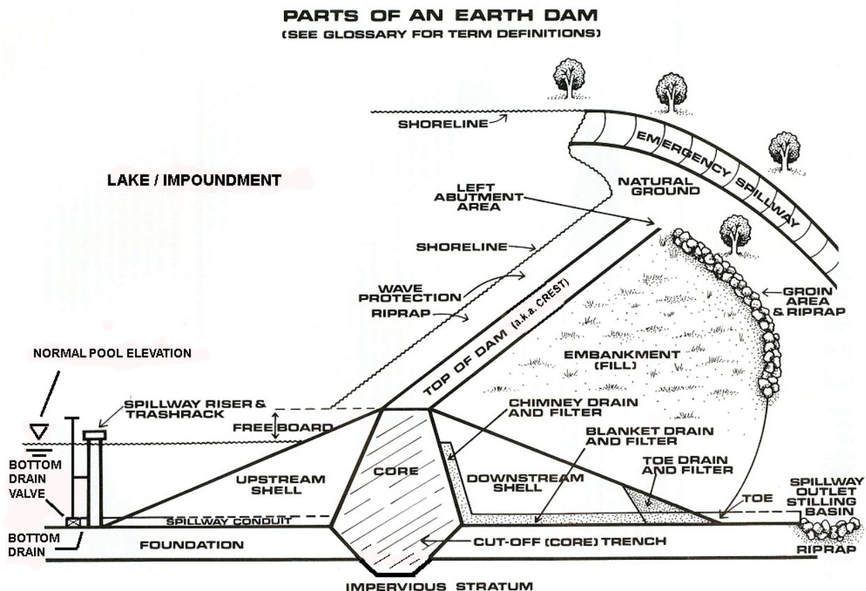
**Figure 2 – Parts of an Earthen Dam (from Dam, Operation, Maintenance, and Inspection Manual – NCDENR Land Quality Section)**
