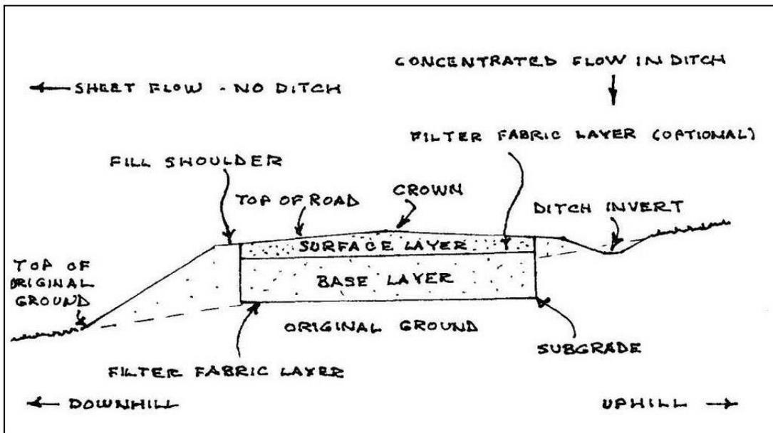
Figure 3 – Typical Road Cross-Section – Canaan, NH Highway Department
