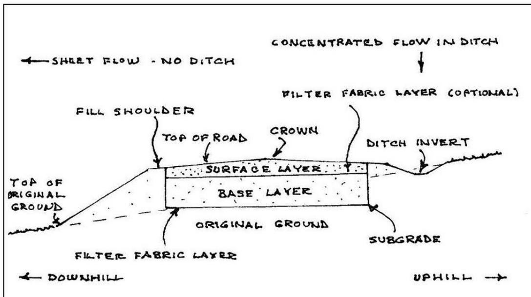
Figure 1 - Typical Road Cross-Section – Canaan, NH Highway Department
