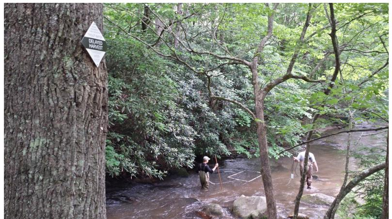
N.C. State University researchers scanning for PIT-tagged trout via a floating antenna (Fixed-antenna arrays were stationed at upper and lower ends of each study reach.) (Photos: Jacob Rash)
