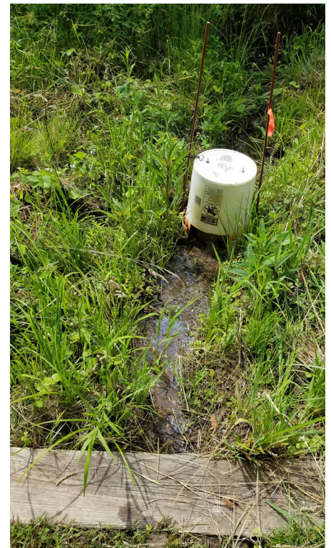
Figure 1. View of a bucket-camera trap set in a rivulet within a mountain bog (Gabrielle Graeter)
