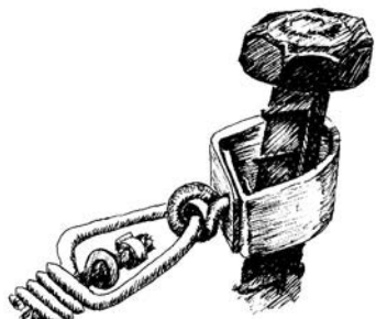
End Swivel with Box Swivel
